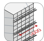
braced + back anchoring b > 600 mm
