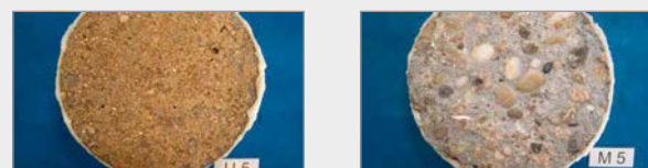
Picture 2: Difference between concrete cores (left side with Zemdrain®, right side without Zemdrain®), after 56 freeze/thaw cycles.
