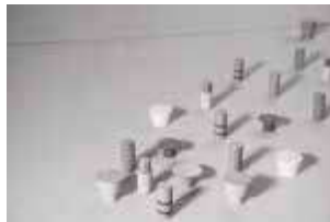
Sealing cones and plugs
