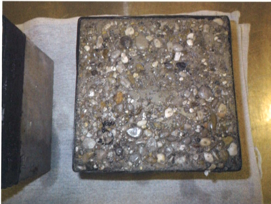
Picture 7: after 28 freeze thaw resistance, strong abgewitterte surface. No damage to the spacer recognizable
