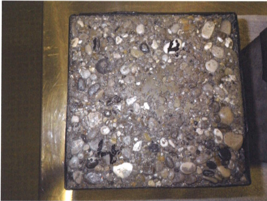
Picture 6: Sample 4 after 28 freeze thaw resistance, strong abgewitterte surface. No damage to the spacers.
