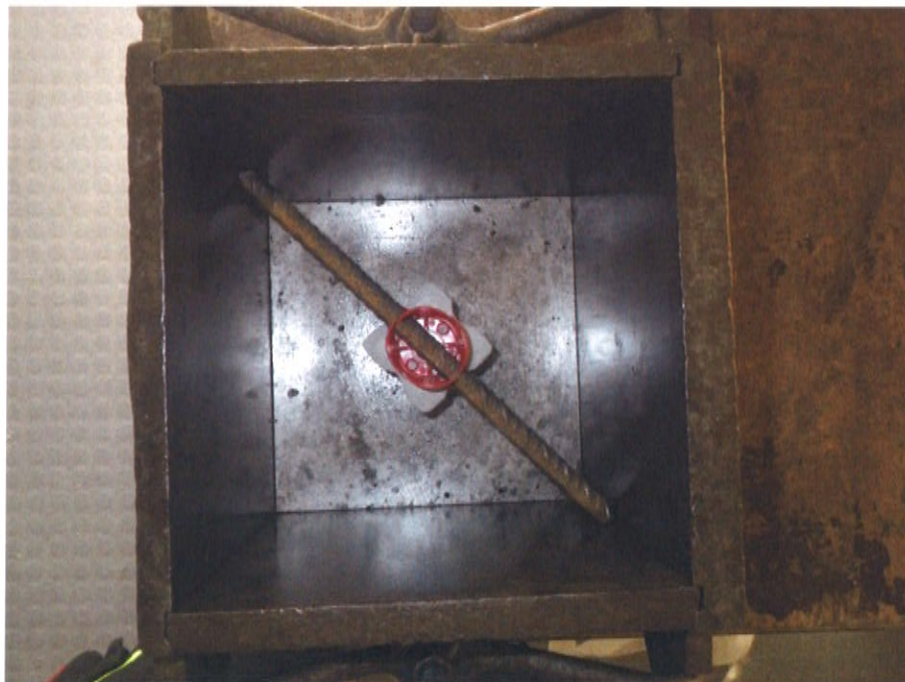
Picture 2: Dice formwork with integrated spacer
