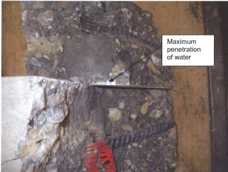
Picture 5 Sample 3 after splitting for measuring the depth of water 3 mm
