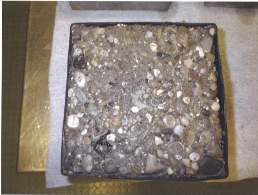
Picture 8: Test 6 after 28 freeze thaw resistance , strong abgewitterte surface. No damage to the spacer recognizable.
