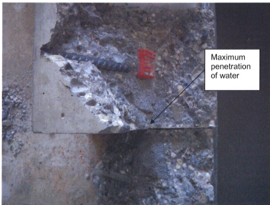
Picture 4: after splitting for measuring the water penetration depth 2 mm
