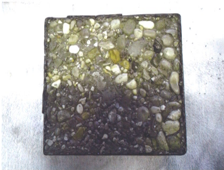
Picture 6: Sample 7 after 28 freeze thaw resistance. Abgewitterte Surface, no damage on the spacers recognizable
