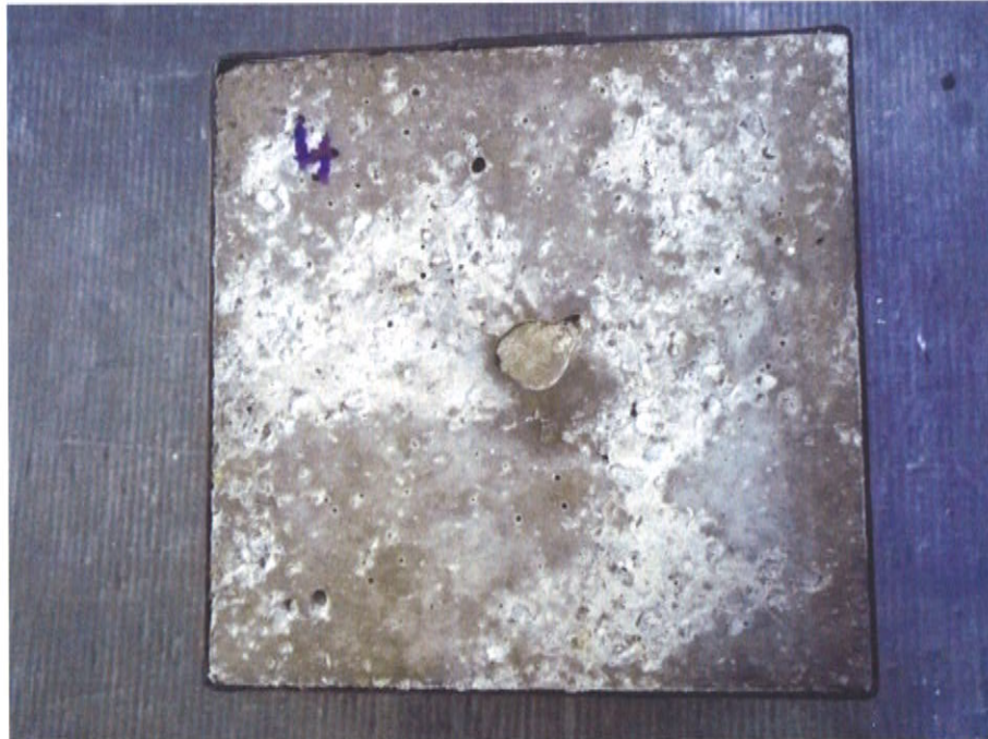
Picture 6: Sample 4 after 28 freeze thaw resistance. Minimum separation on spacers recognizable
