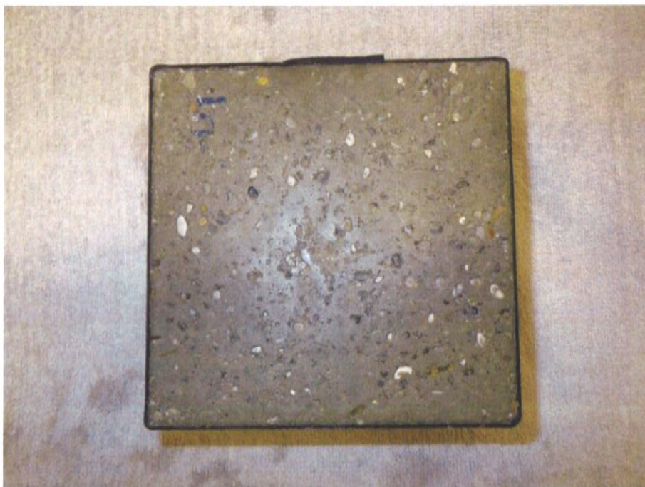
Picture 7: Sample 5 after 28 freeze thaw resistance, abgewitterte surface. No damage on the spacer recognizable
