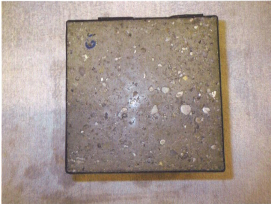
Picture 8: Sample 6 after 28 freeze thaw resistance, abgewitterte surface. No damage on the spacer recognizable.
