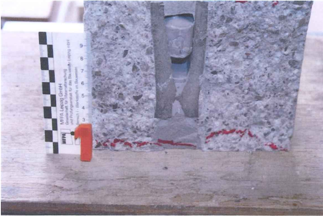
Photo 1: Series C 'FRANK fibre-reinforced concrete distance tubes – MR 22 sealed with one fibre-reinforced concrete plug St220020 and one 3 cm fibre-reinforced concrete sealing cone FBVKZ22T, sample 1
