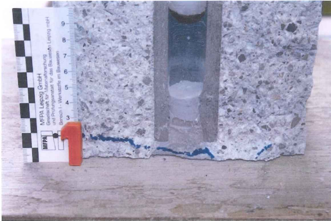
Photo 1: Series B 'FRANK fibre-reinforced concrete distance tubes – MR 22 with one fibre-reinforced concrete plug and one fibre-reinforced concrete sealing cone FBVKZ22, sample 1
