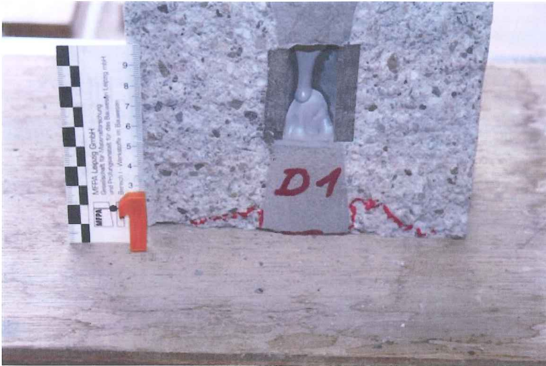
Photo 1: Series D 'FRANK fibre-reinforced concrete distance tubes – MR 22 each sealed with one 5 cm sealing cone FBVK22T50, sample 1
