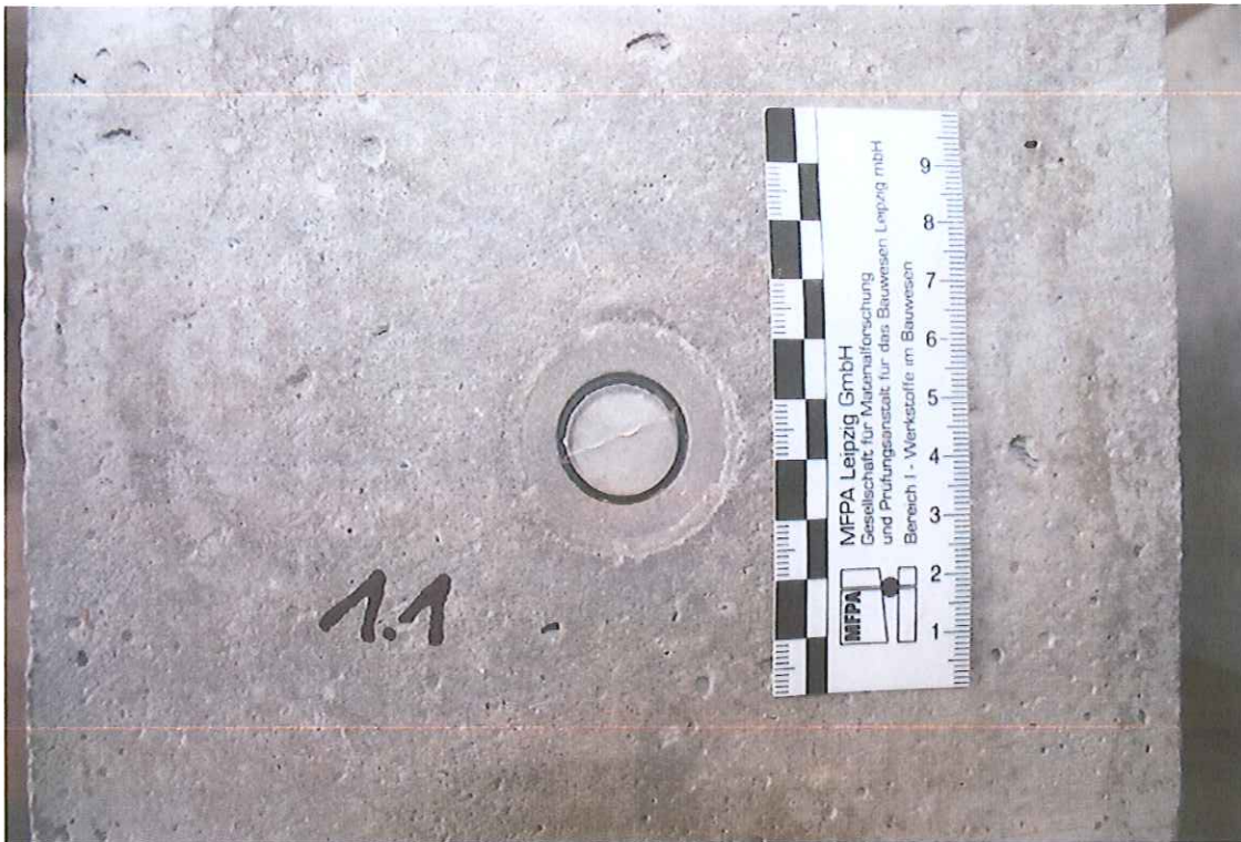
Figure 1: The sealing plug of test specimen 1.1 after the pressure test
