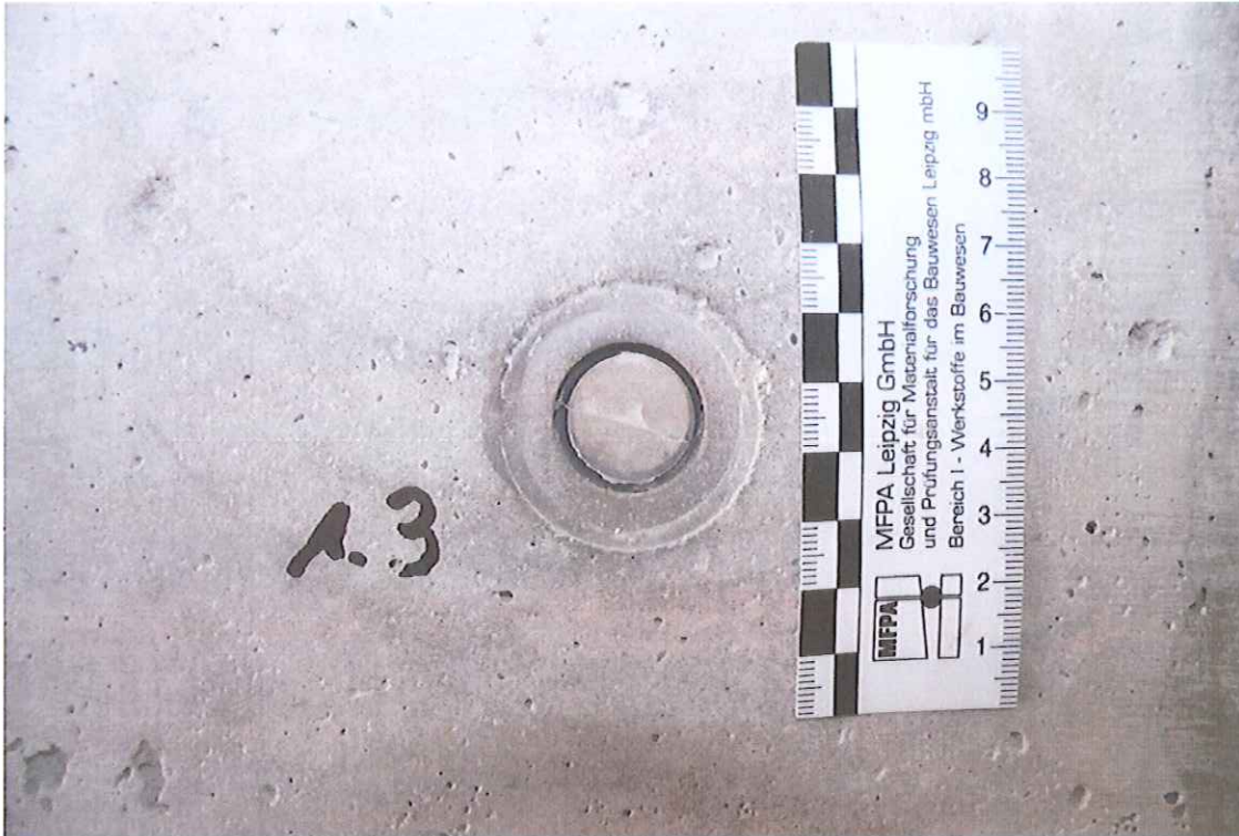
Figure 3: The sealing plug of test specimen 1.3 after the pressure test
