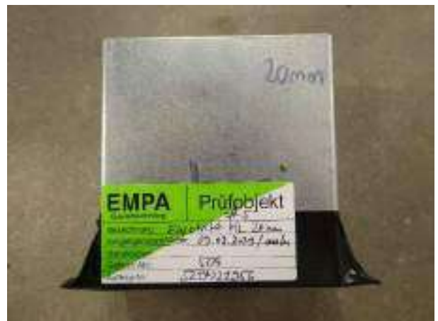
Figure 11: Stair landing bearing Egcopal SPH with 20 mm elastomer bearing (with old description on the test label)
