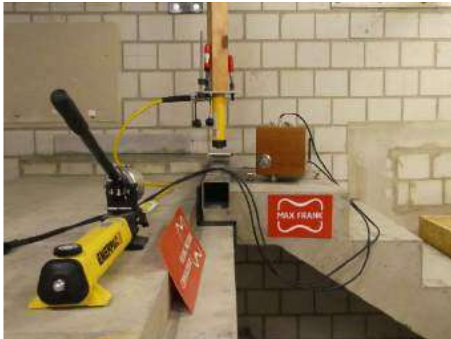
Figure 37: Hydraulic ram for applying additional loads on the stair flight (configuration 1)
