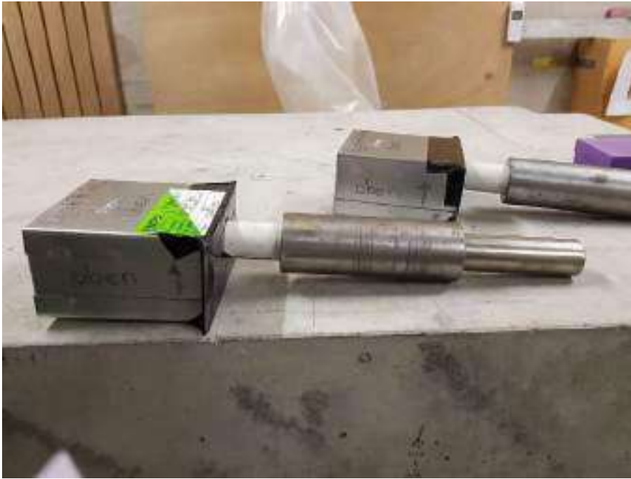
Figure 22: Stair landing bearing Egcopal SP with 20 mm elastomer bearing with dowel and adapter sleeve before installation
