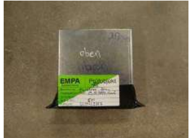
Figure 13: Stair landing bearing Egcopal SP with 20 mm elastomer bearing (with old description on the test label)
