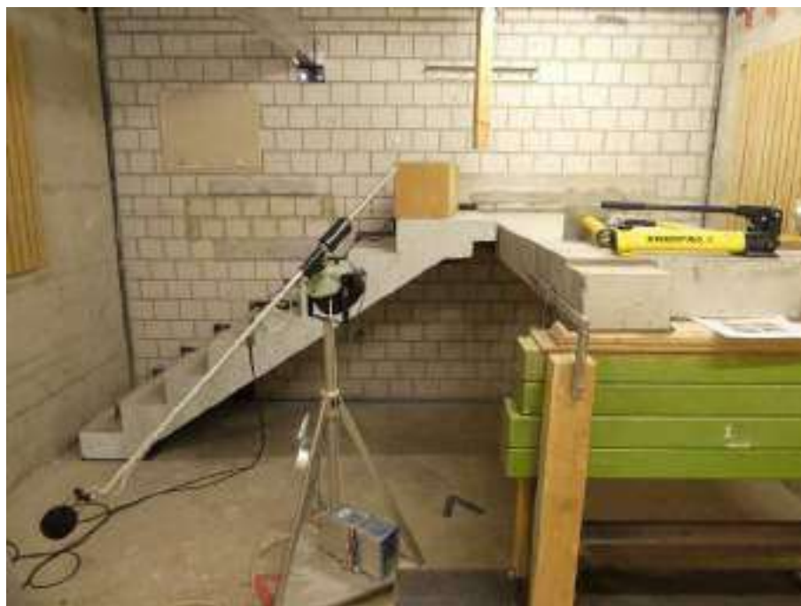
Figure 29: First arrangement for testing staircase bearings and landing bearings (configuration 2)
