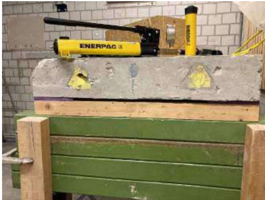
Figure 30: Auxiliary wall as bearing for reference stair landing 1 for testing stair landing bearings (configuration 2)
