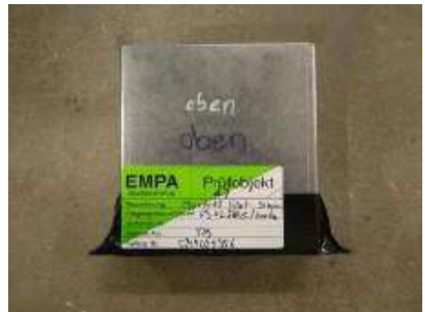
Figure 15: Stair landing bearing Egcopal SP light with 20 mm elastomer bearing (with old description on the test label)
