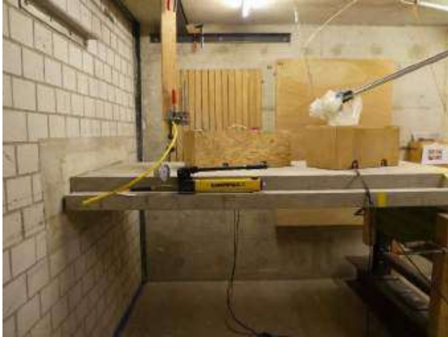
Figure 42: Overview of the installation situation and tapping machine positions on the stair landing
