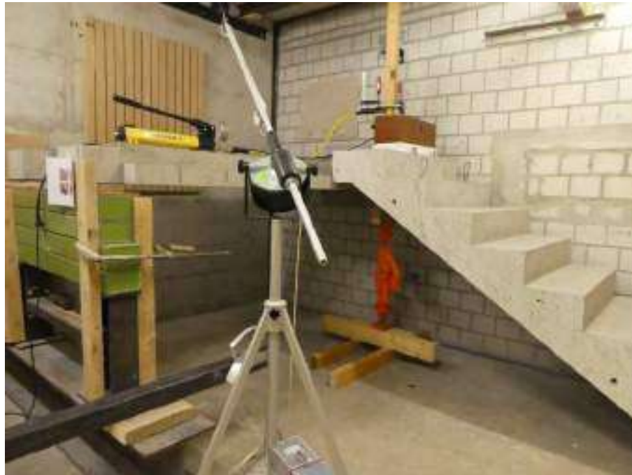
Figure 28: First arrangement for testing staircase bearings (configuration 1)
