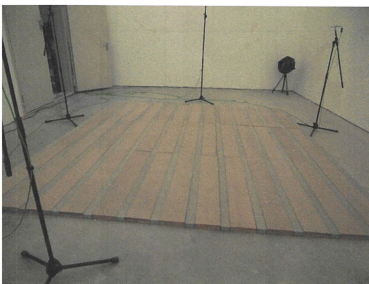
Image appendix 2: test setup 2 in the reverberation room of the HFT Stuttgart.
